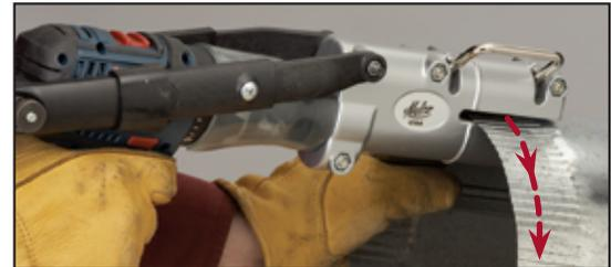
The rotation of the meshing teeth on the adjacent gears drives the metal out the right side of the tool head. Use the throat depth line as a guide to control the length of the crimp.
