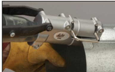
Use the crimper depth adjustment lever, in the down position, to open gears for easy insertion and removal of metal.
