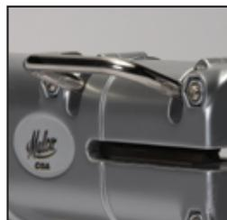
Start the crimp to the left of the duct or pipe lock-seam. With the lever in the up position, the maximum crimping depth is factory set for optimal results in 26 to 28 gauge (0.56 to 0.48 mm) galvanized steel. Back off the lever for lighter metals or re-adjust the maximum crimp, per operators manual, for heavier metals. A clutch in the gear mechanism prevents damage to the crimper attachment if seams are encountered that exceed crimper capacity.
