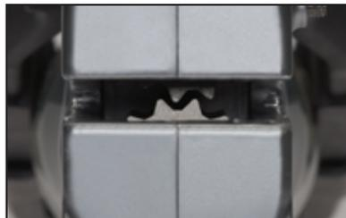
The narrow point of entry in the face of the tool prevents fingers from entering the gears that produce the crimp.
