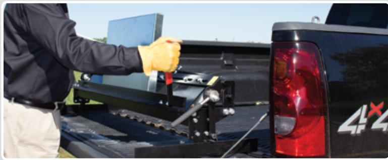
For fabricating *shop-quality pans and boxes*, on the job, the Malco 48 in. (1.2 m) “Pan Style” Mini-Brake *quickly breaks down and goes to work with you!*
