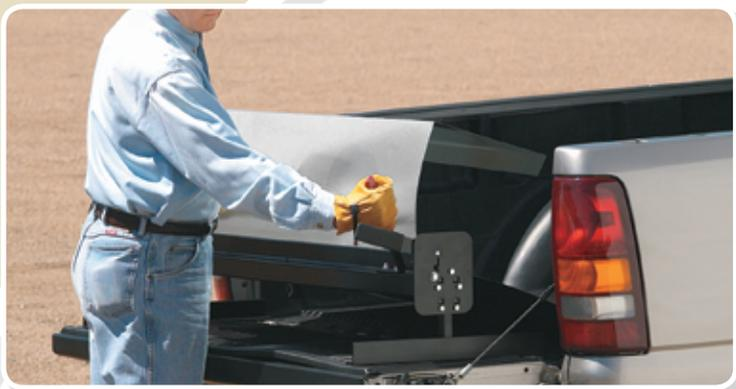
Makes bends to 135 degrees in galvanized sheet steel up to 22 gauge (0.86 mm). A beefed-up 5/16 in. (7.9 mm) plate steel apron and 48 in. (1.2 m) metal width capacity makes the Mini Brake ideal for fabricating plenums or large transitions at the job site.
