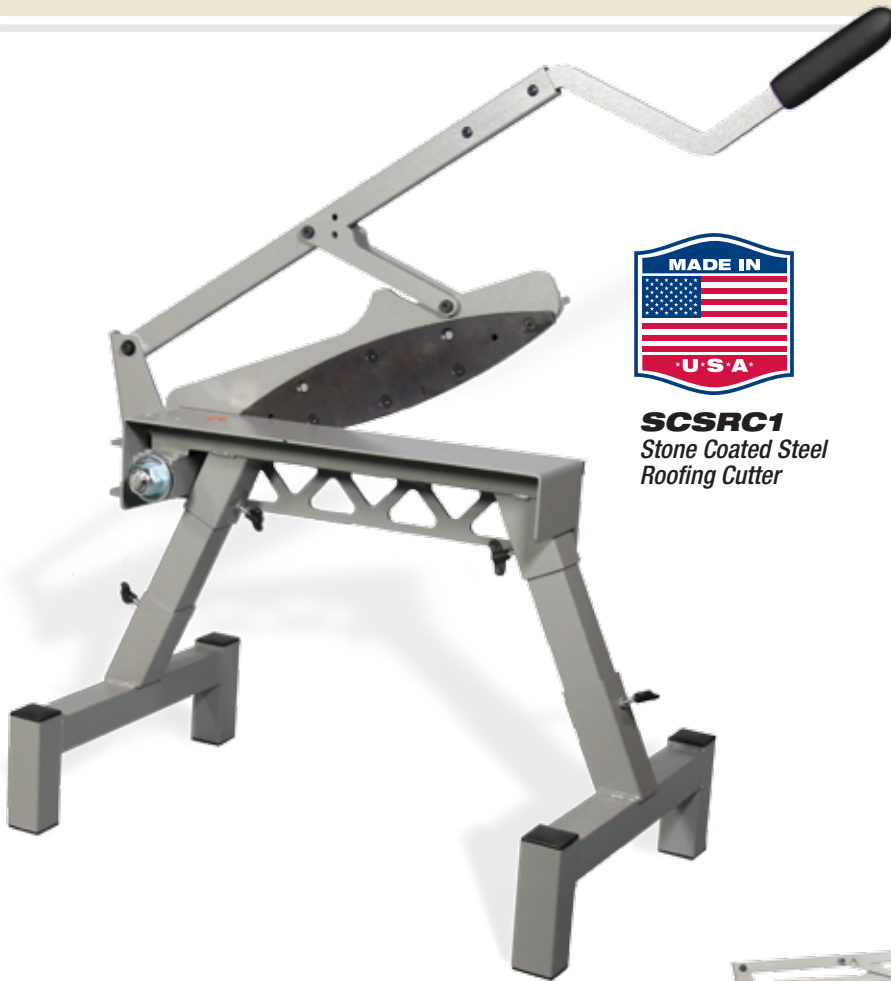
The steel shingle, including lock seam, is cut in an easy, steady motion. The shearing action has a "wiping" effect on the shingle's zinc coating that seals cut edge to resist rust.
