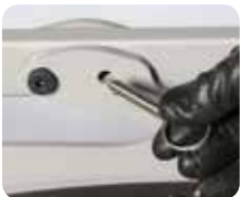
With blade lock-pin in place, this cutter is safe to carry on to the job site.
